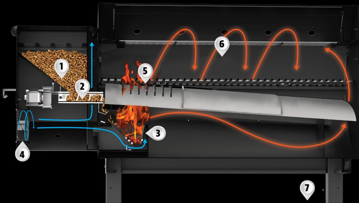
1. TRAMOGGIA DEL PELLET 3. ALLOGGIO FIAMMA 5. GRIGLIA CON FIAMMA 7. SECCHIELLO PER IL GRASSO
